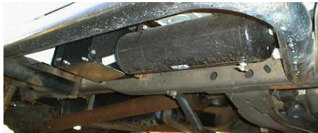
Car-mounted compressed air tank
